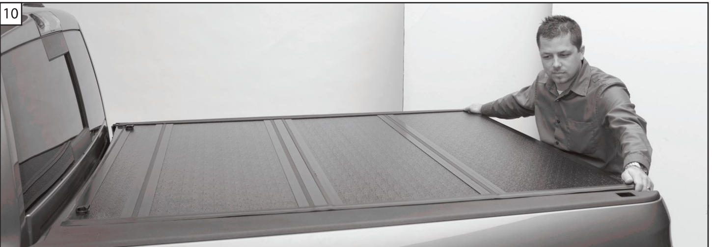
10. Test the rear latching assembly for smooth operation as this is the best indicator of the cover being positioned correctly. Be sure the latches on both sides are engaging with the cover mounting rail.
