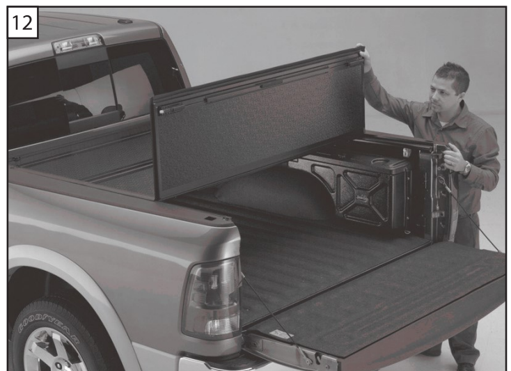
11 & 12. Once the cover is located correctly, fold the cover to the open position. Pull the release cables on the rear panel to release it from the side rail. Take care to fold it gently so the position of the cover is not disturbed.
