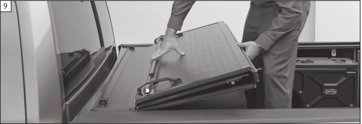
9. Carefully unfold the cover. Position the cover so it is centered side to side and front to back on the truck bed.
