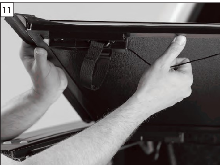
11 & 12. Once the cover is located correctly, fold the cover to the open position. Pull the release cables on the rear panel to release it from the side rail. Take care to fold it gently so the position of the cover is not disturbed.
